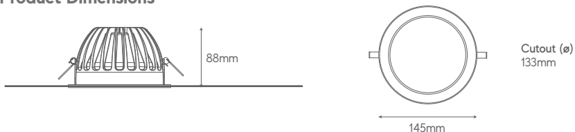
Die-Cast Aluminium Body
